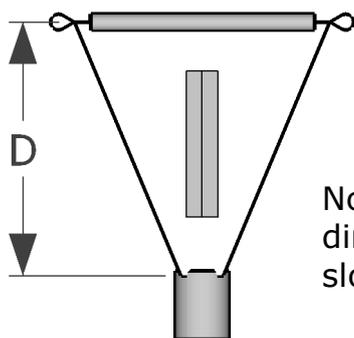
Note: "D" is the vertical dimension, not the angled slope measurement
